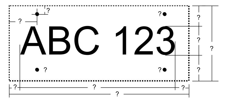
If mounting holes are required, specify choice of a) 8 mm round, or b) 1/4"x3/4" slot. Circle appropriate size.
