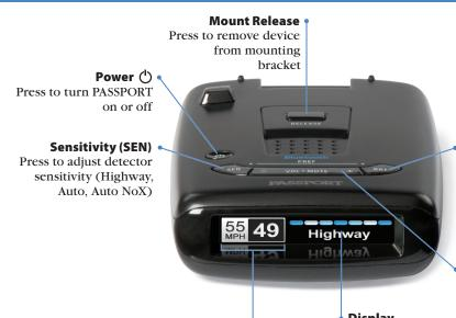
Brightness (BRT) Press to adjust display brightness (Min, Med,
