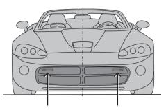
For optimal performance, sensors need to be facing straight forward (or backward, if installing optional rear sensors), level to ground. Make sure that each sensor is parallel with the road (using supplied bubble level).
