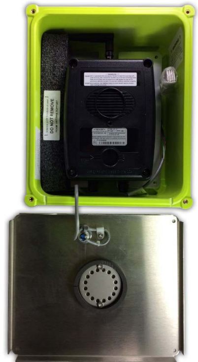
XT-Series case with metal faceplate removed
