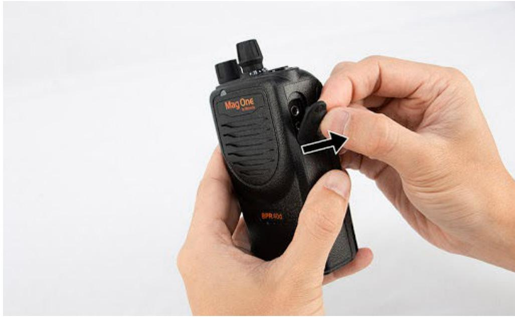
**Postrequisites:** Replace the dust cover when the universal connector is not in use.
