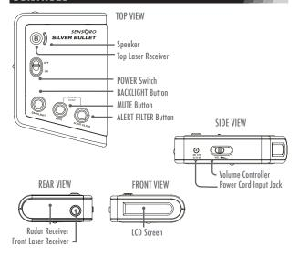
The SILVER BULLET RX7500 can be easily installed on your windshield, visor, or dashboard. Each location has its own installation hardware and requirements.
